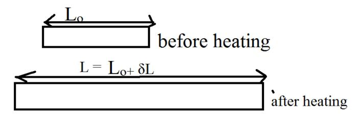
When a solid is heated its length increases then the expansion is called linear expansion. Consider a rod of length  $L_0$ , when the rod is directly heated, the increase in its length  $\Delta L$  is proportional to its original length  $L_0$  and change in temperature  $\Delta T$
